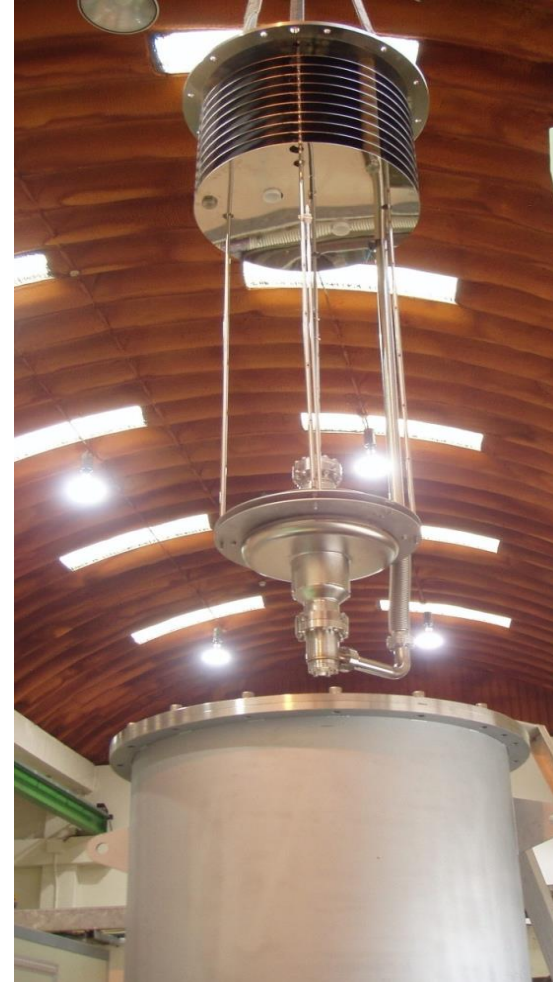
Cryostat for Vertical Test
