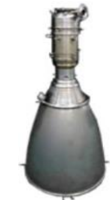
Combustion Chamber (For 10Ton Grade)
